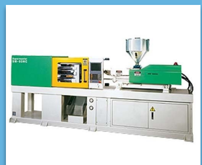
Thermoplastic Moulding 150 Ton in Moulding Shop
